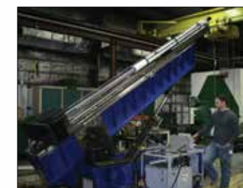
Convertible Test System 20,000 lb load - 100" CC
